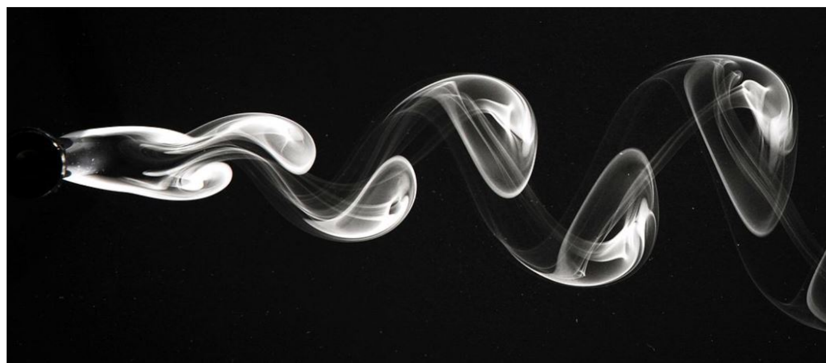
Figure 1: Figure shows flow separation after a blunt body with cyclical motion following low pressure regions
