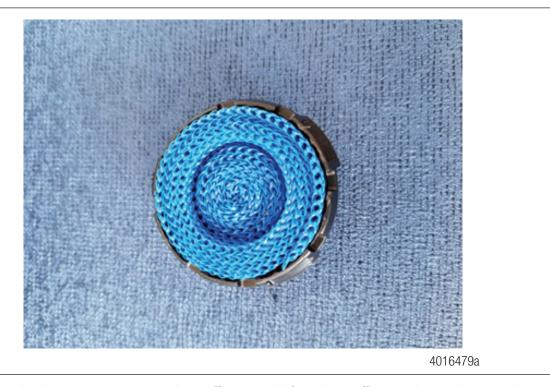
5. If further cleaning is necessary, remove the muffler material from the muffler housing and un-wrap it. Use water to clean it as needed then wrap it back up and reinstall it in the muffler housing.
