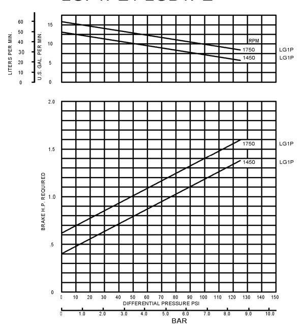
**NOTE:** Blackmer Characteristic Curves are based on Brake Horsepower (BHp). To determine Motor Horsepower, drive train inefficiencies must be added to the BHp.
