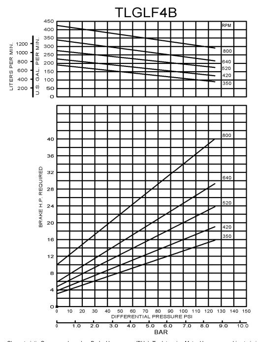
**NOTE:** Blackmer Characteristic Curves are based on Brake Horsepower (BHp). To determine Motor Horsepower, drive train inefficiencies must be added to the BHp.
