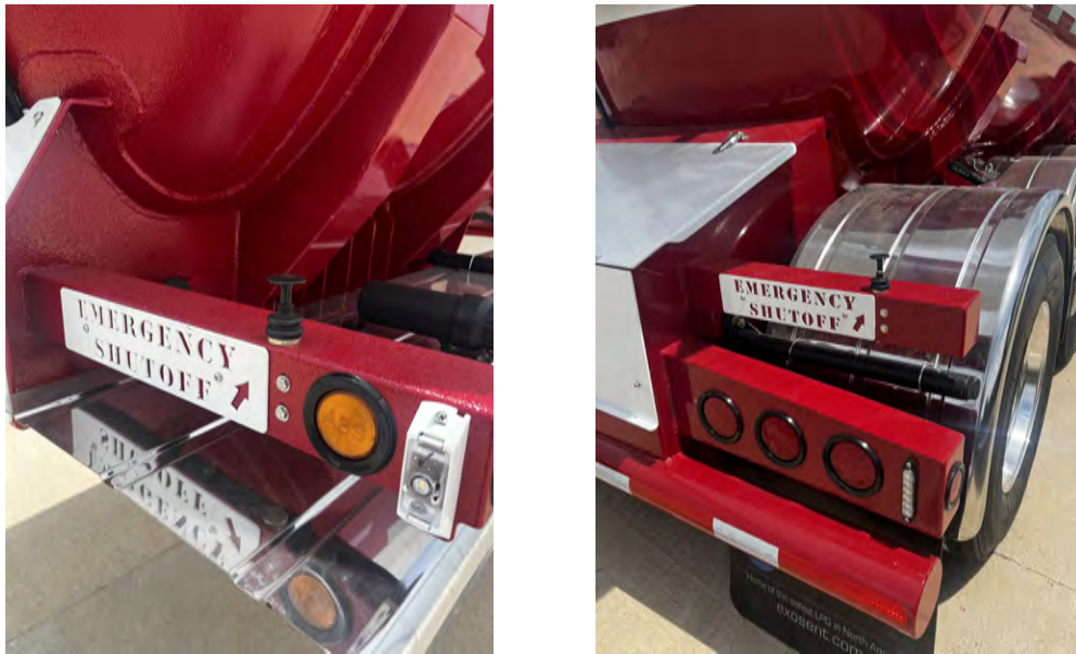
Figure 9: Left: Emergency Shut off valve front. Right: Emergency Shut off rear.
