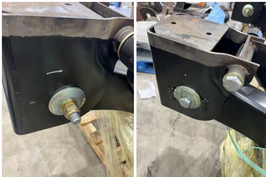
Figure 11: Left: Suspension hanger with bushing bolt as seen from inside chassis frame. Right: Bushing bolt (bottom left) as seen from outside of chassis frame. This bolt is also used to adjust suspension alignment, see suspension alignment routine below.
