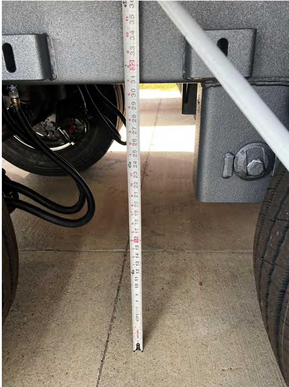
Figure 17: The Figure shows the way to measure trailer ride height from the ground to the bottom of chassis. The current figure shows the ride height in bag dump condition.
