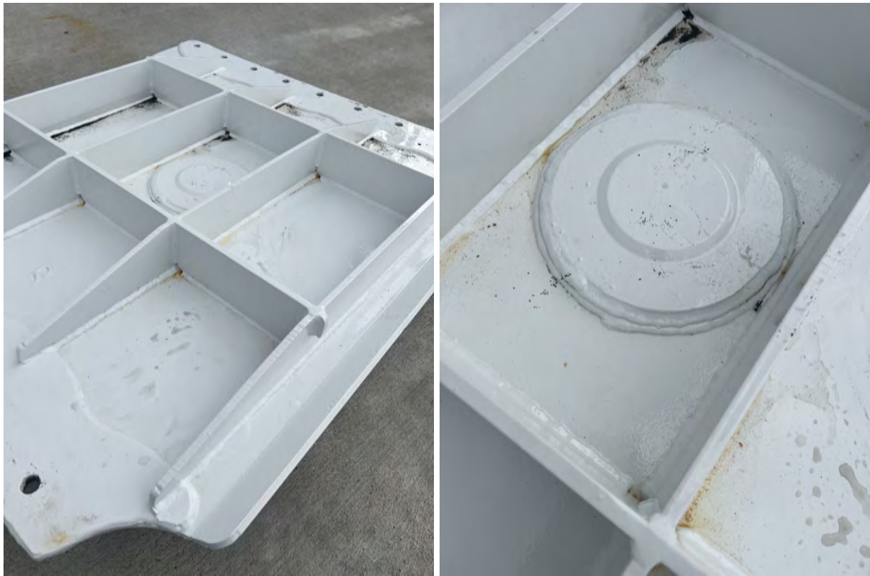
Figure 3: Upper Coupler structure, left: upper coupler welded ribs, Right: upper coupler King Pin welds
