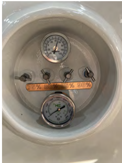
Figure 12: Spitter valves are shown in the well with percentage limits below the valves. The pressure gauge is located on the bottom and the temperature gauge is located on top.
