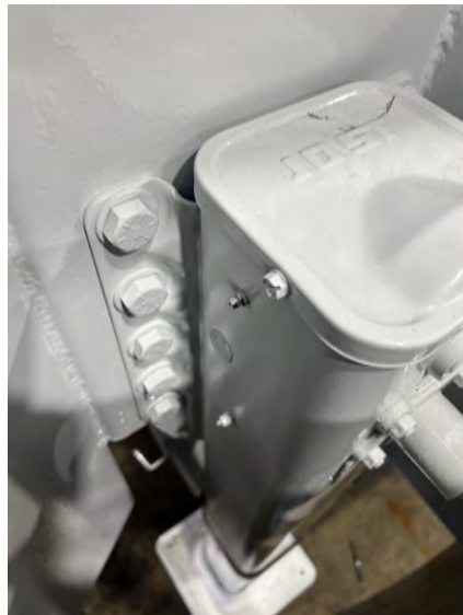
Figure 13: Shown typical landing gear with grease zirc fittings located on the side of the leg
